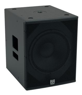
The X115 is a very compact subwoofer designed to augment the low frequency performance of BlacklineX Series full-range systems. It comprises a long excursion 15" (380mm)/3" (75mm) voice coil driver in a bass reflex enclosure and can be used singly, stacked or flown via integral M10 inserts. Four large ports contribute to a reduction in air noise at high output levels.
